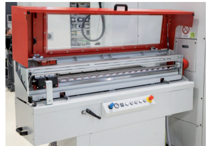
Operating panel. The operating buttons and the diameter adjustment are located on the front side of the SL 1200. If required, the loader can easily be moved 400 mm to the left.
