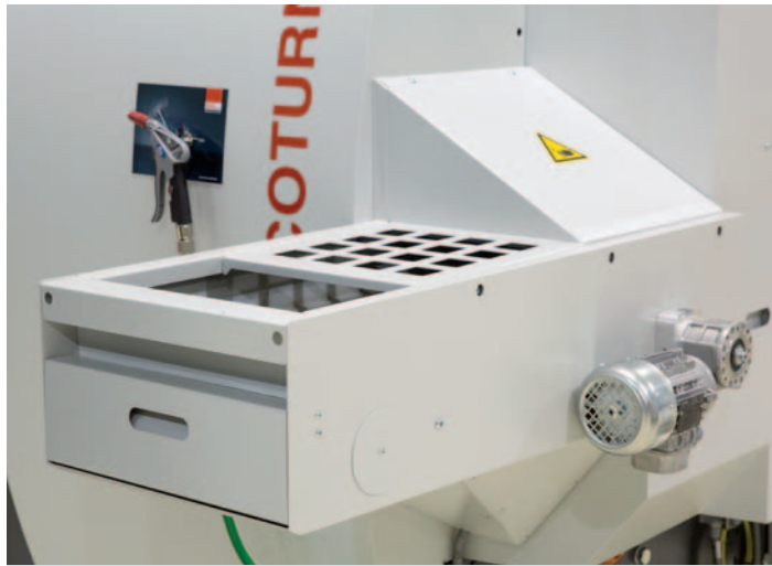
Finished parts conveyor. The finished parts catcher places the finished parts onto a collector belt. Since the belt is clocked, the parts – which are often very complex – are kept from falling on top of each other.
