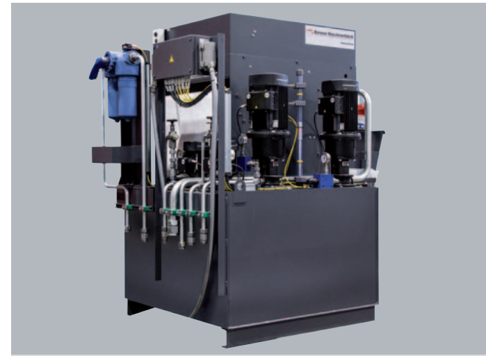
Belt filter system. If required, it is possible to install an optional 600-litre belt filter system with 25 bar high-pressure coolant pumps. It increases both the cooling emulsion volume and the coolant's service life.
