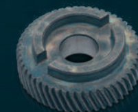
Gear (Bore hard-turned)
