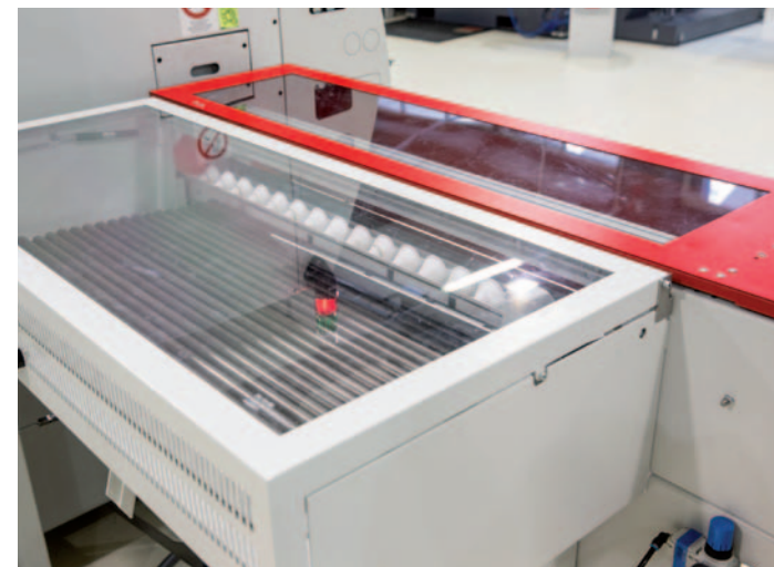
Material support. The material support attached to the back of the SL 1200 features a surface of 560 x 1210 mm and allows stocking a large number of bars. This allows for unmanned production. To ensure compliance with the safety guidelines, the material support is covered by a hood.
